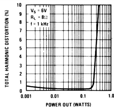
Figure 6. Total Harmonic Distortion vs Power Out
