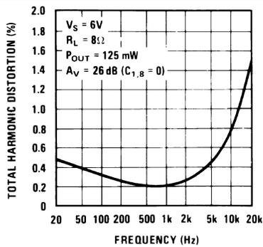
Figure 5. Total Harmonic Distortion vs Frequency
