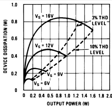
Figure 9. Device Dissipation vs Output Power
