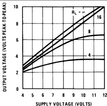
Figure 3. Output Voltage vs Supply Voltage
